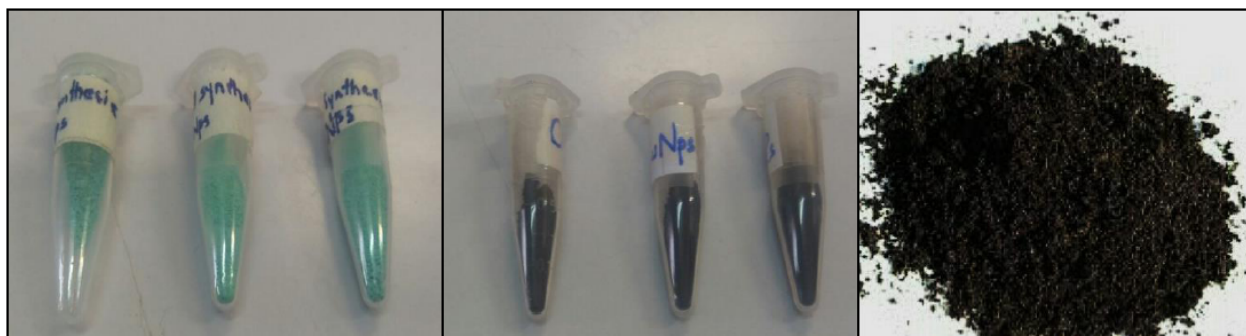
Fig. 1: Precipitates obtained after centrifugation of reaction mixture; black CuO NPs obtained after annealing at 400°C
