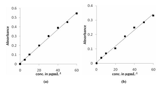
Figure 2. Calibration curves for a) DOX and b) DOT
