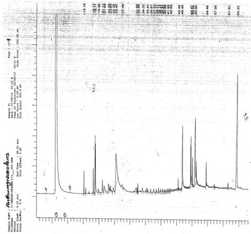
Gas chromatogram of volatiles in the hydrodistilled oil of Sudanese *Anethum graveolens* fruits analyzed by GC-MS. GC-MS, gas chromatography-mass spectrometry.
