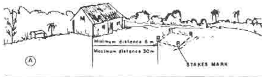
Fig. 30. PIT LATRINE (a) LOCATION OF PIT SITES (b) WOOD BASE (c) BLOCK OR BRICK BASE
