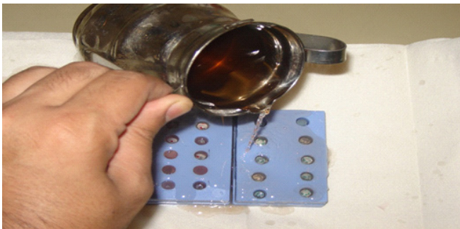
Fig 1: Introducing molten wax to the surface of the specimens in the silicone mould
