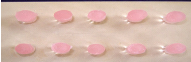
Fig 2: Waxed acrylic rods held in a stone mould for dewaxing
