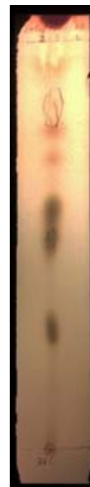
Fig. 3: TLC profile of Soxhlet methanol extract using solvent system of Chloroform: Methanol: Acetic acid (3:1:1)
