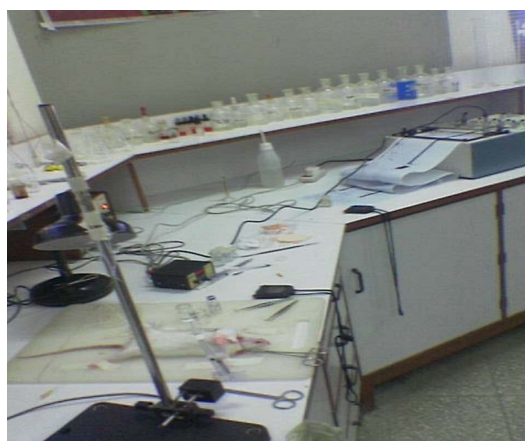
Fig. 2: The blood pressure transducer connected with the left carotid arterial cannula and recorder
