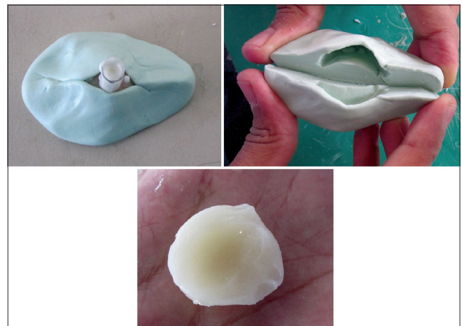
Figure 2a: Fabrication of the trial wax shell
