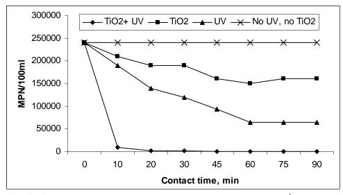
**Fig. 3:** Effect of irradiation time on *Coliform* removal:  $TiO_2 = 0.8$  gr L<sup>-1</sup>, pH=7.0
