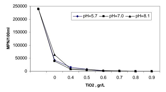
Fig. 2: Effect of TiO<sub>2</sub> concentration and pH on *Coliform* removal as MPN/100 ml:
