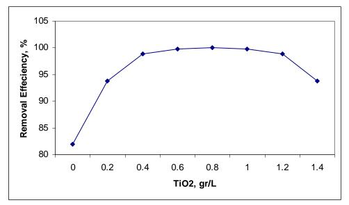
Fig. 4: Effect of TiO<sub>2</sub> concentration on *Coliform* removal as MPN/100 ml:
