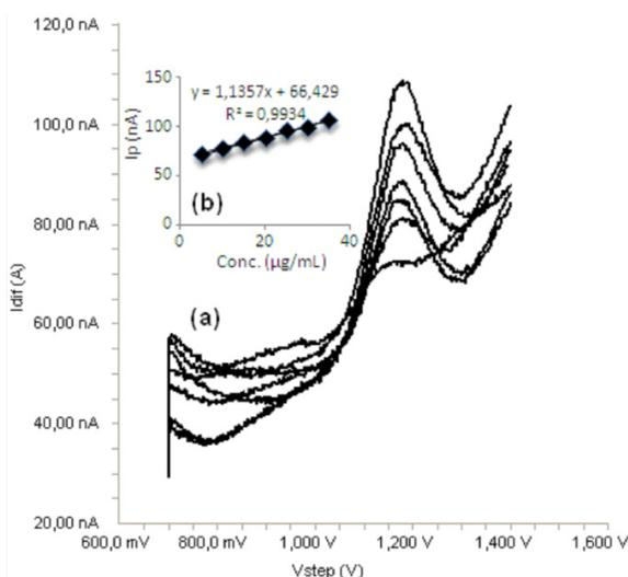
**Figure 7.** a) Square wave voltammograms for different concentrations of bosentan in acetonitrile solution containing 0.1 M TBAClO<sub>4</sub> (5, 10, 15, 20, 25, 30 and 35 µ
