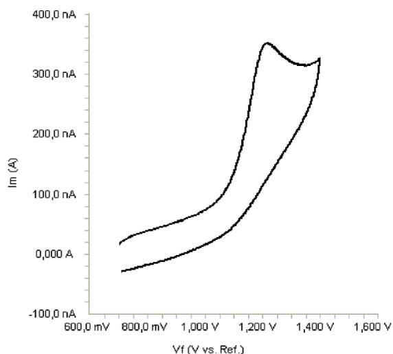
**Figure 2.** Cyclic voltammogram for the oxidation of 20 µg/mL bosentan in acetonitrile containing 0.1 M TBAClO<sub>4</sub> at Pt disk electrode, scan rate: 0.1 V s<sup>-1</sup>.
