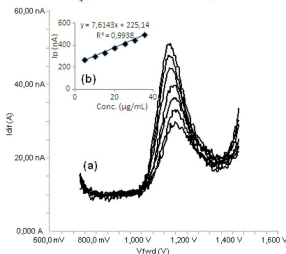
**Figure 8.** a) Differential pulse voltammograms for different concentrations of bosentan in acetonitrile solution containing 0.1 M TBAClO<sub>4</sub> (5, 10, 15, 20, 25, 30 and 35 µ
