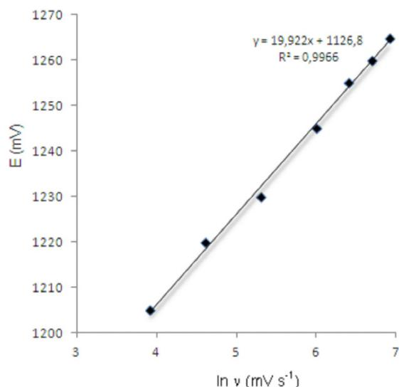
Figure 5. Dependence of anodic peak potentials of voltammetric peak for the oxidation of 20 µg/mL bosentan on the scan rate.
