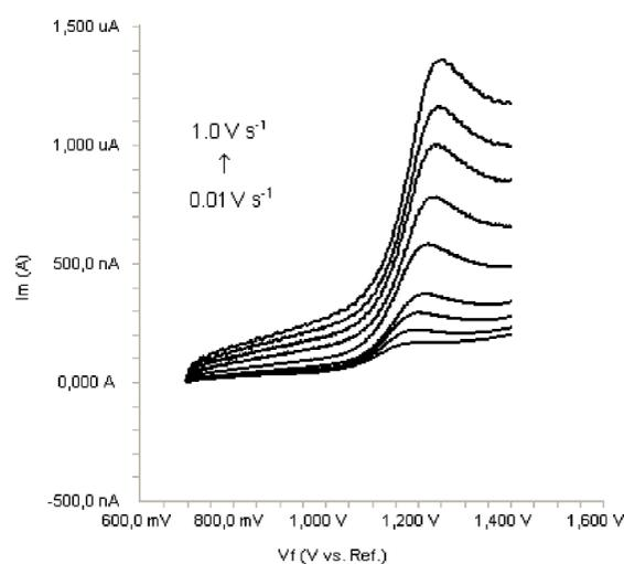
**Figure 3.** Linear sweep voltammograms for the oxidation of 20 µg/mL bosentan in acetonitrile containing 0.1 M TBAClO<sub>4</sub> as a function of scan rate.
