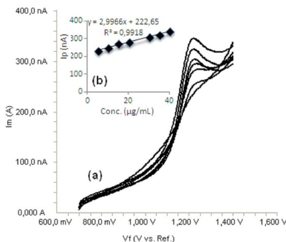
**Figure 6.** a) Linear sweep voltammograms for different concentrations of bosentan in acetonitrile solution containing 0.1 M TBAClO<sub>4</sub> (5, 10, 15, 20, 30, 35 and 40 µ
