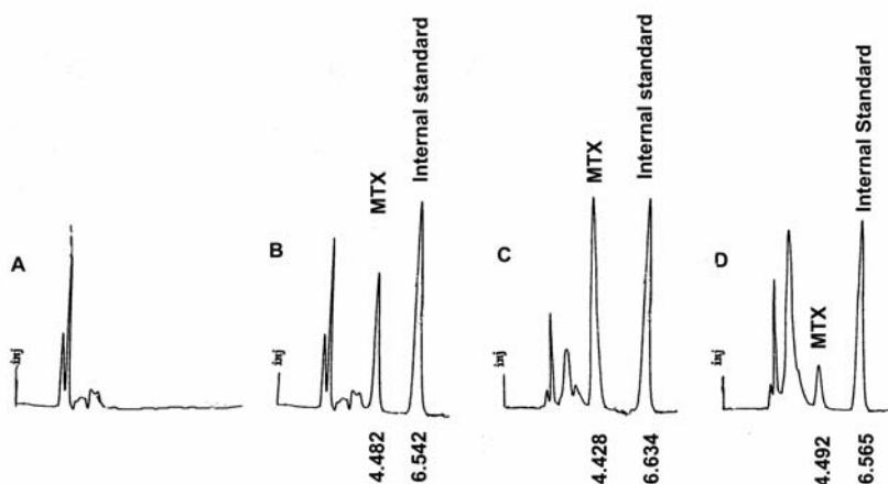
**Figure 1.** Chromatograms: A-human blank plasma, B-MTX standard (25  $\mu$ M), C-Patient plasma sample at the end of a 4-h infusion of 2 g/sqm of MTX, D-patient plasma sample 7 hours after the end of a 4-hours infusion of 2 g/sqm of MTX. (detector sensitivity: 0.005 a.u.f.s; injection volume: 10  $\mu$ l)
